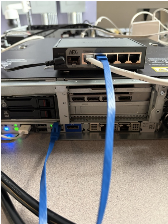
(c) HPE blade iLO connection to the router using the blue cable.
