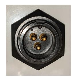
Locate the notches on the female end of the power pigtail. Align them with the depressions in the AC power boundary connector, press in, and lock into position by screwing in the twist lock.
